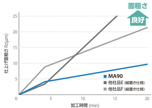
切削条件 : Vc = 200 m/min, ap × ae = 1 × 37.5 mm, fz = 0.1/0.12 mm/t, Dry S50C ø50 (6/7枚刃) BT50
