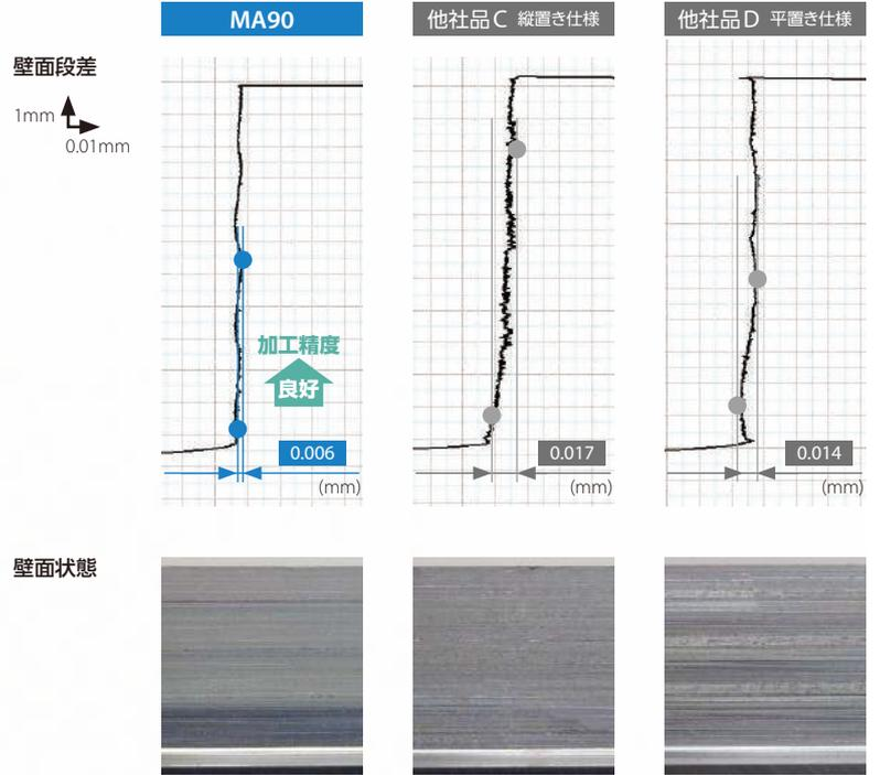
切削条件 : Vc = 150 m/min, ap × ae = 3 × 5 mm 4/パス, fz = 0.1 mm/t, Dry S50C ø20 (3枚刃) BT50
